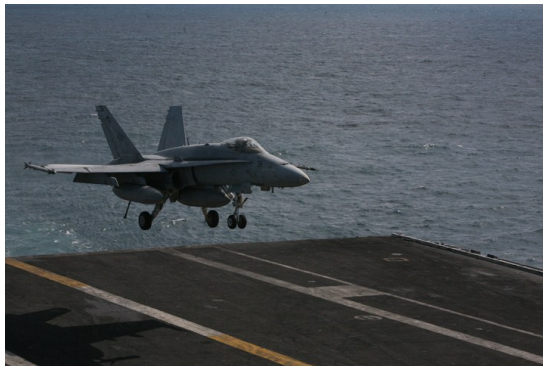
A F/A-18C comes in for an arrested carrier landing aboard the USS John C. Stennis (CVN 74) after completing a training mission for Northern Edge 2009. (U.S. Air Force photo/Marine Corps Sgt. Zachary Dyer)
