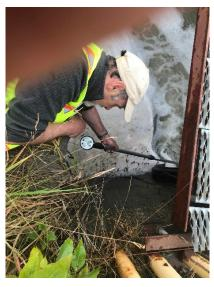
Measuring flow at the JBER-E Outfall 1 culvert (drainage from Cherry Hill)
