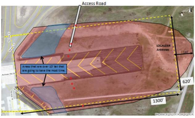
= Area that is getting plowed down to 3' or less of the ground level of the antennas
