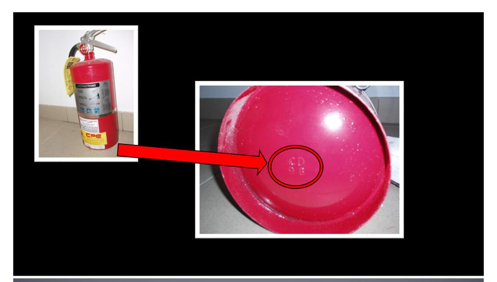
If no maintenance label present, you must use the year of manufacture to determine the next maintenance. The year of manufacture may be stamped on the bottom of the fire extinguisher or on the bottom outside edge of the cylinder, with a 2-digit number signifying the year.
