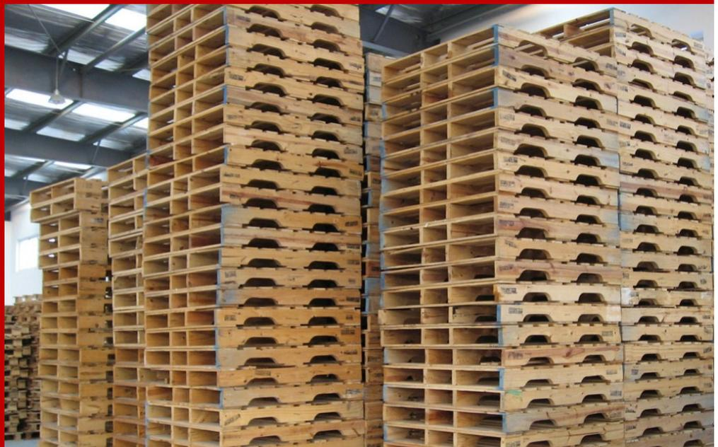
Improperly stored or improperly protected pallets can add a significant fuel load to any facility and can also overwhelm the sprinkler system. Stacking idle pallets in piles is the best arrangement of combustibles to promote rapid fire spread and is one of the greatest challenges to sprinklers.
